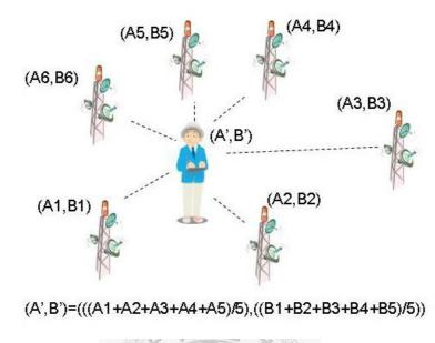
Fig. 2. Centroid Positioning (the coordinate of beacons is a prior knowledge)
