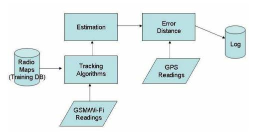
Fig. 6. System Architecture (Tracking)
