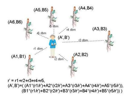
Fig. 3. Weighted Centroid Positioning
